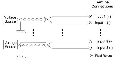
An external source must be provided to power input transceivers.
